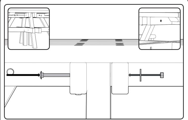
9. Insert the M10 x 180mm coach bolt (Item 4) through the table top support and the tops of the legs. Take care to insert the fixing through the small hole and not the larger counter bore hole. Secure with a washer (Item 5) and nyloc nut (Item 6). Use a 17mm socket wrench to tighten the nuts.
