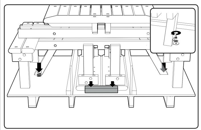
2. Using the hand drill or screwdriver unscrew the fixings holding the timber blocks supporting the seat assemblies during transit. Remove the 2 x wingnuts holding the table legs to the pallet.
