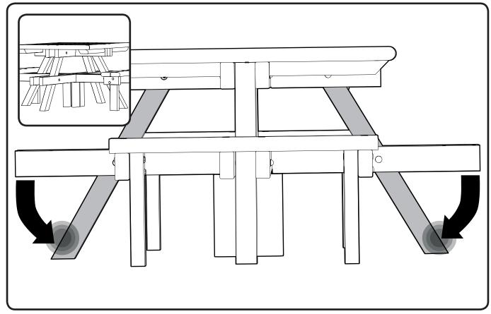
8. Pivot the legs downward from the crossbar and leg assembly. Align the fixing holes between the top of the leg and the underside of the table top frame by tapping the base of each leg with the mallet until they line up. Remove the support blocks.
