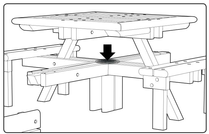
7. Ensure the crossbars are fully engaged by gently tapping the crossbar and leg assembly down with the mallet directly above the support blocks until the tops of the crossbars are level.
