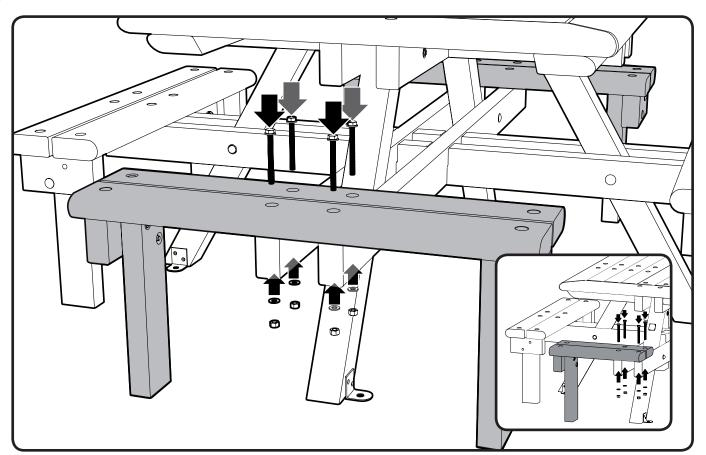
11. Insert  $4 \times M10 \times 130$ mm bolts (Item 9) through the seat and crossbar (mallet may be required). Secure in position using the washer (Item 5) and nyloc nuts (Item 6). Use  $2 \times 17$ mm socket wrenches to tighten all fixings. Repeat the process for the seat opposite.
