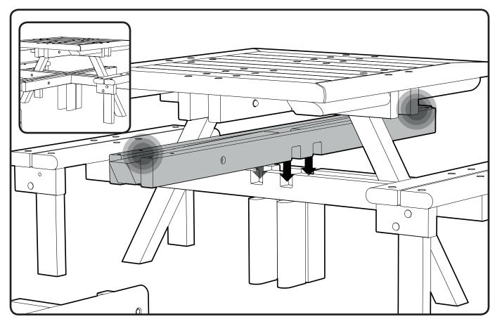
6. Feed the crossbar and leg assembly (Item 1) through the table pack assembly and slot it into the corresponding halving joints of the fitted lower crossbar. Take care to orientate the crossbar and leg assembly the correctly with the halving joints facing the downward.
