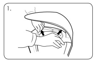
Lift the two sack bands upwards.
