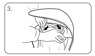
Push the sack bands down to trap the sack between the bands and the sack ring, clamping it in an open position ready for use.
