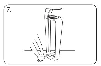
Tighten the bolts into the ground using a 17mm spanner or socket set.
