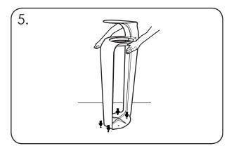
Reposition the bin over the drilled holes. Place the washers [ITEM 3] onto the bolts [ITEM 2].
