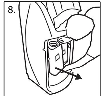
8. Using two hands, slide one of the reservoirs towards you holding the handle in one hand. **IMPORTANT:** This may be heavy (less than 10kg) so take care when removing.
