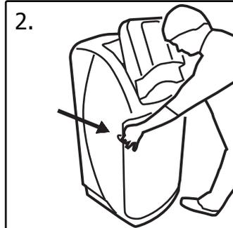
2. Lift both catches on either side of the door at the same time to release it.
