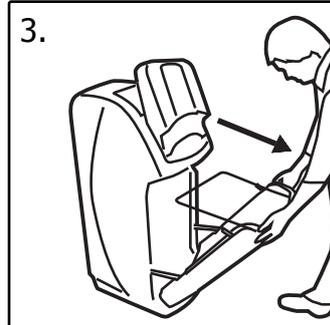
3. Pull the door forwards so that it rests on the retention straps.
