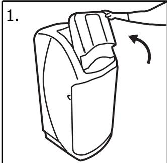
1. Lift the tray shelf upwards so that it is resting against the aperture.
