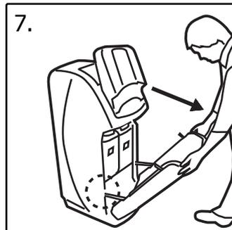
7. Open the door of the bin, steps 1-3. Should you need to gain better access to the reservoirs, the door can be removed by unhooking the straps (see circle above).
