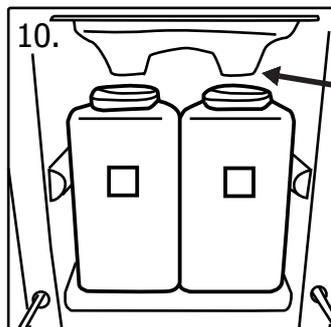
10. After emptying the reservoirs, replace by standing them on the reservoir holder. Ensure the handles are at the front for ease of emptying and the warning stickers are facing towards the door.
