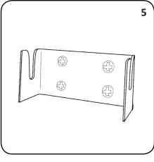
Tighten the Screw with the Screwdriver and repeat for all 4 fixings points securing the Cup Stacker Bracket to the wall.
