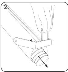
Using the Stainless Steel ring, open the Quick Release Mechanism to remove cups.
