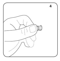
Push 4 x ITEM 2 into the 4 drilled holes. Tap the plugs lightly with the Hammer to ensure they are flush with the wall surface.
