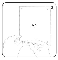
Place ITEM 1 against the wall 60mm above the top of ITEM 5. Mark 4 fixing points on the wall through the 4 holes in the A4 Foamex Sign, ensure the sign is horizontal and centrally straight.
