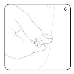
Place ITEM 4 against the wall aligning the 4 holes with the 4 wall plugs, Thread through one of the SCREWS and tighten with the Screwdriver.
