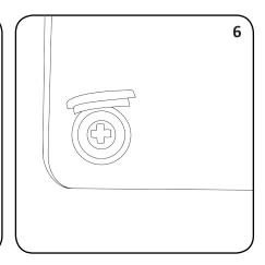
Place the A4 Foamex Sign against the 4 fixings holes and thread one of the Screw fixings into the wall plug. Fit all 4 fixings, using the Screwdriver to tighten.
