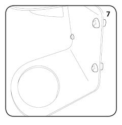
Repeat step 6 for all 4 fixing points Place ITEM 5 onto the Cup securing the Drip Tray Bracket to the wall.
