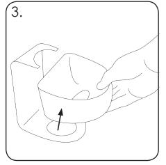
To empty or clean the Drip Tray, remove the Drip Tray from the Drip Tray Bracket.
