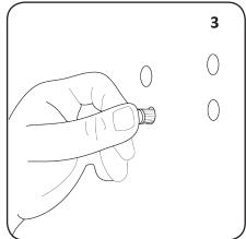
Push 8 x ITEM 2 into the 8 drilled holes. Tap the plugs lightly with the Hammer to ensure they are flush with the wall surface.
