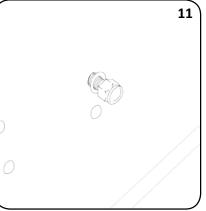
At the top of the bin body, align ITEM 7 over the fixing holes on the outside of the Nexus 100. Place ITEM 1 through one of the 4 fixing holes. On the inside of the Nexus 100 Body place ITEM 3 onto ITEM 1 and fit ITEM 8 onto ITEM 1. Tighten the nut with the Spanner and Allen Key.
