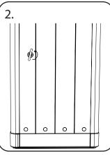
Turn key in the keyhole anticlockwise until it stops.
