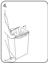
Reposition elasticated sack band to secure plastic sack.
