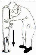
3. Insert bollard stem into sprocket and twist until bollard drops to engage.
