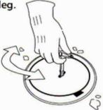
3. Lift blanking cap with key.
